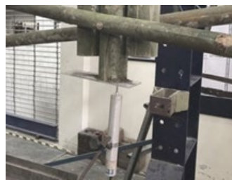
Fig. 27. Truss decrease with displacement transducer
