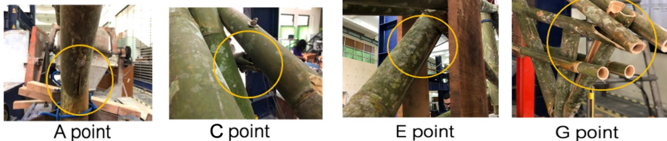
Fig. 32. Breakage points detail after experiment
