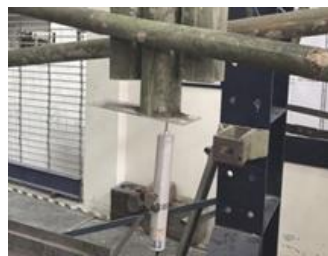
Fig. 27. Truss decrease with displacement transducer
