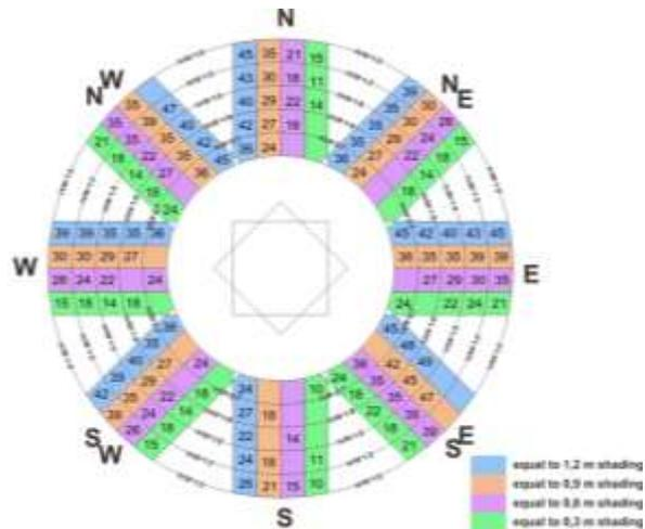
Fig. 9. The Effective Shadow Angle on each Side Based on H/W Ratios
