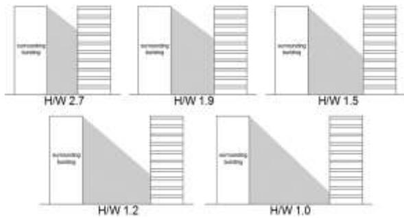
Fig. 3. Shadowing Illustration of the Surrounding Buildings
