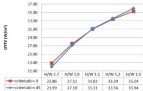
Fig. 4. OTTV Value Based on the H/W Ratio
