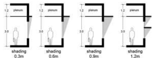
**Fig. 2.** Shadowing Illustration of Shading Device on Typical Floor of ‘Stand-alone’ Building Condition
