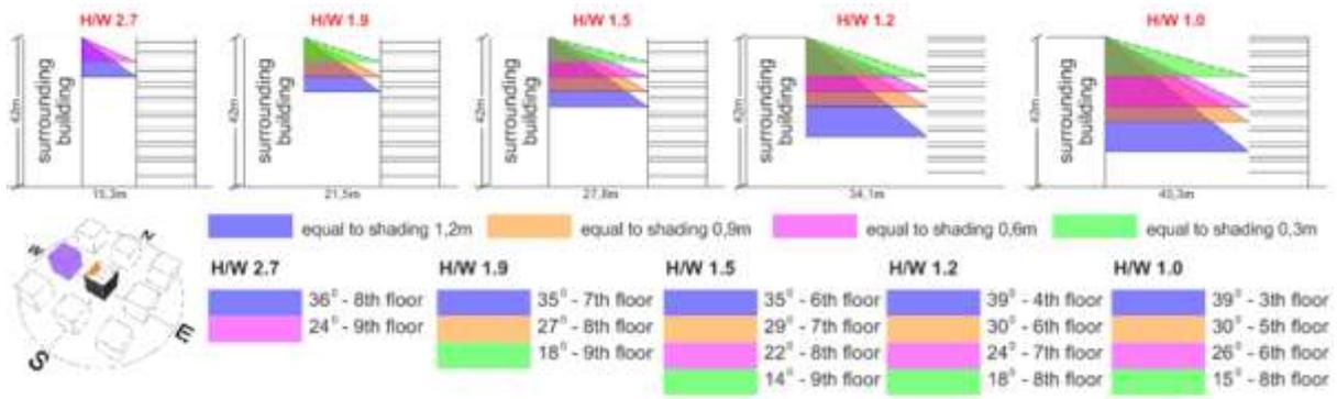
Fig. 7. The Effective Shadow Angle Based on the H/W Ratio (Western orientation)
