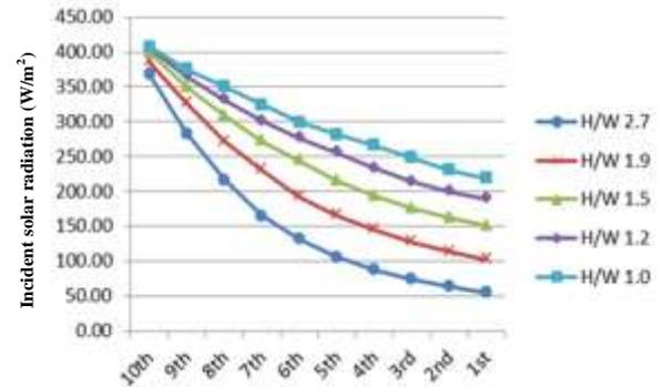
**Fig. 6.** Incident Solar Radiation on the Western Orientation
