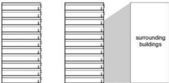
Fig. 8. The Use of Effective Shadow Angle for Minimizing the Use of 1,2 m Shading up to 8th floor (right) Compared to the Condition of Shadowing in Stand-alone Building (left)
