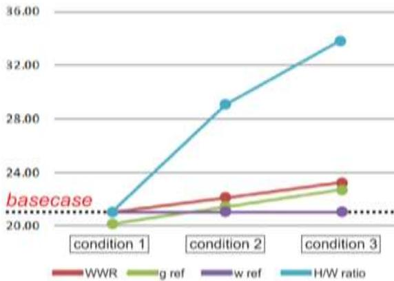
**Fig. 5.** OTTV Based on Changing Surrounding Building Variables Compared to Basecase Conditions (orientation 0°)
