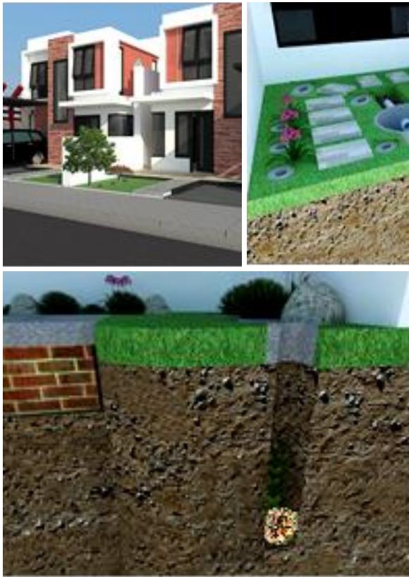
Figure 5. Layout of biopore absorption hole in the front yard (left), in the backyard (middle) and the detail design (right)
