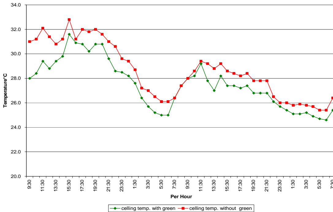
Figure 5. Profile of green roof ceiling surface temperature and bare roof ceiling surface temperature
