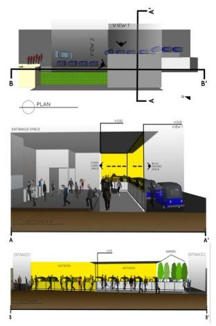
Fig. 4. Plan and sections of Manggarai Station that show solid-void elements.
