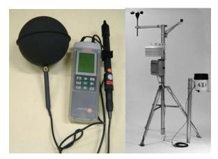
**Fig. 1.** Handheld Equipment Testo 445 and Weather Station HOBO (Source: author and gayeontech.co).
