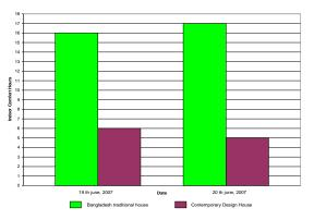
**Figure 7.** Profile of Indoor comfort hours in both B.T.H and C.D.H within 24 hours.
