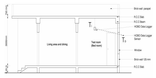
Figure 4. Section of typical contemporary designed house and the position of data logger and sensor.
