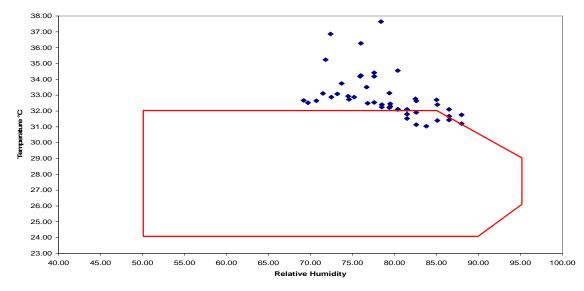
Figure 6. Plotting of the indoor space temperature and the indoor relative Humidity of C.D.H within summer comfort zone.
