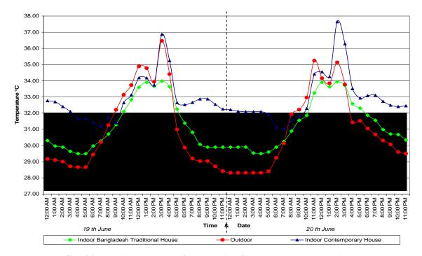
Figure 5: Profile of indoor air temperature of B.T.H (taken from Rumana, (2008)) and C.D.H compare to outdoor air temperature with identified comfort zone.
