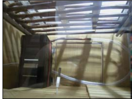
Figure 9. Condenser coils unit inside the model acting as evaporator to reduce the model temperature
