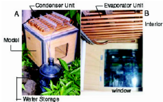
Figure 4. (A) The scale model & condenser copper coils on top. (B) The evaporator copper coils inside the scale model.
