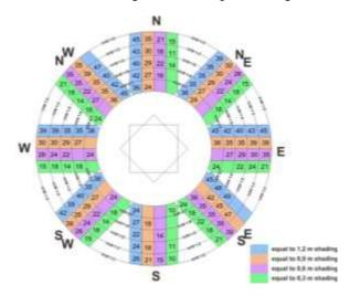
Fig. 9. The Effective Shadow Angle on each Side Based on H/W Ratios
