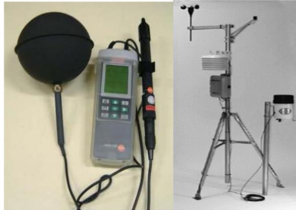
Fig. 1. Handheld Equipment Testo 445 and Weather Station HOBO (Source: author and gayeontech.co).
