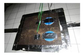
Figure 4. Attaching Thermocouples & Heat Flux
