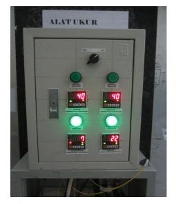
Figure 11. Temperature Controller running on Hotbox Equipment
