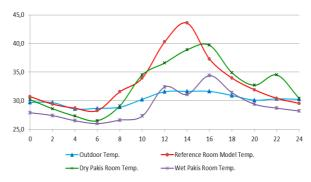
Figure 12. The Room Temperature of Reference model, Dry and Wet Pakis-Stem-Blocks
