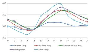
Figure 8. Dry Pakis-Stem-Blocks Model Thermal Performance
