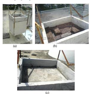
**Figure 5.** The Researched Models (a) and Pakis (Picas)-Stem-Blocks covered on Mode (b)), Reference Model with flat concrete rooftop (c), (author, 2010)
