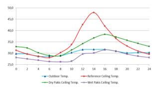
**Figure 11.** The Ceiling Concrete Temperatures of Reference model, Dry and Wet Pakis-Stem-Blocks
