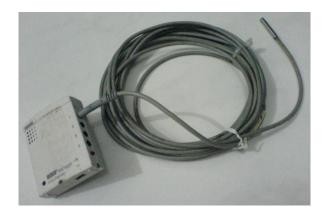
**Figure 6.** HOBO U Family Data Logger and External Water or Soil Sensor, (author, 2010)
