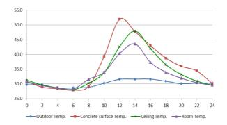
Figure 7. Reference Model Thermal Performance
