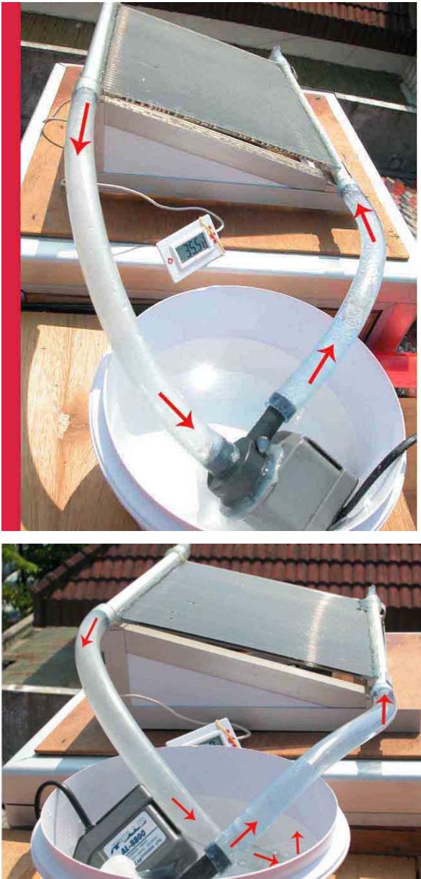
Fig. 6. The water flushing systems on polycarbonate skylight (closed system on the left)
