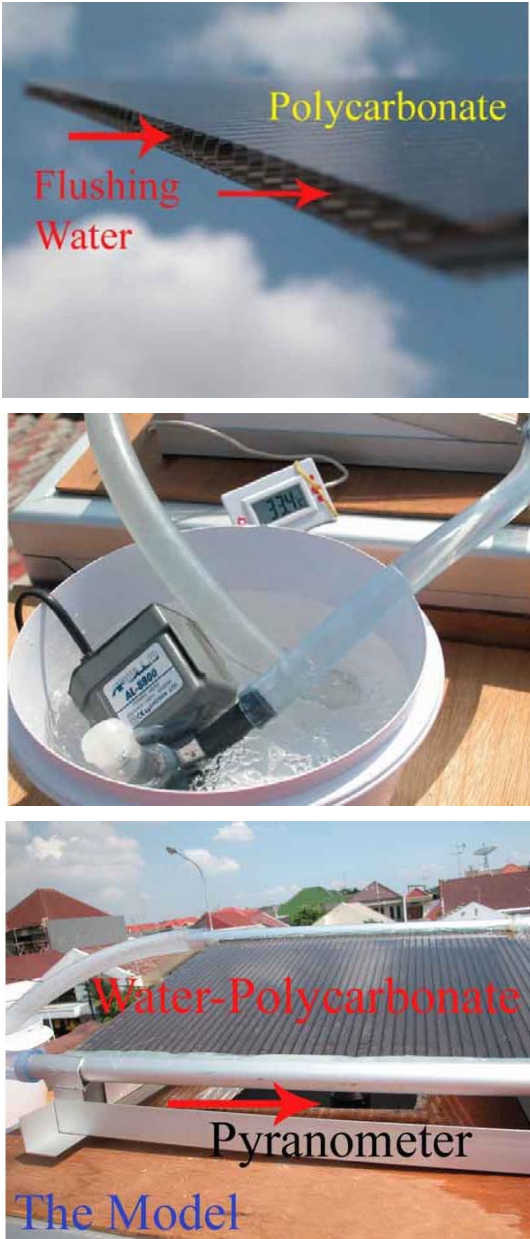
Fig. 5. The water-polycarbonate skylight device and measurement tools
